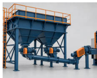
BOILER FUEL FEEDING
